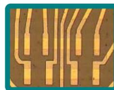
Medical application with 14µm lines and spaces
