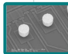
Medical application with 70µm-pitch flip chip
